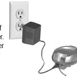
2. Place the mouse's charging contacts on the charger's contacts to charge the batteries.
